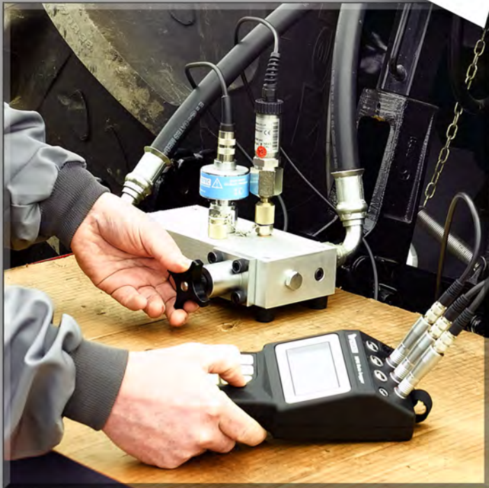
Faultfinding on a tractor with the HPM460
