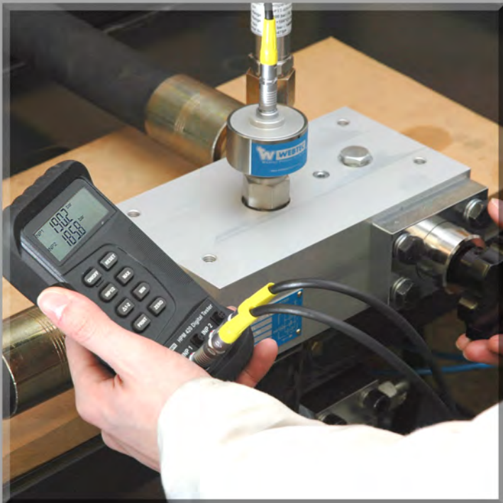
Testing pump flow and pressure with the HPM420
